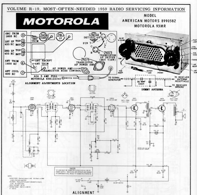
Connect an output meter across the speaker voice coil. Set tone control to high and volume to maximum. Attenuate signal generator output to maintain 1.3 volts on output meter to prevent overloading the receiver.
